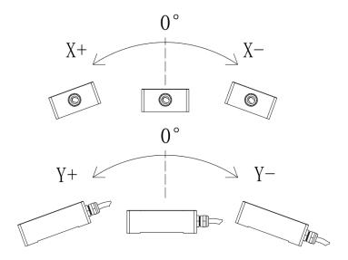
ZCT2xxM-LBS-AV-H5-460x should be installed vertically:
